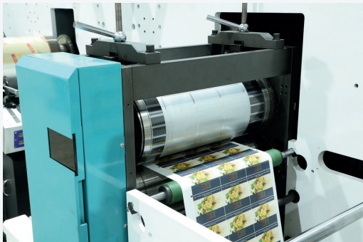
Semi-rotary die cutting unit with three servo driver control system.
