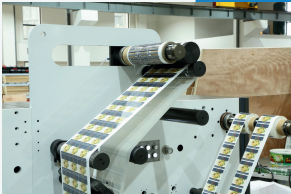
Snowball waste collector suitable for various shapes of labels.
