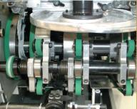
Disk Attachment Rotary Feeder with Disk ttachment. Used for oound or folded piece where the orientation requires feeding from the open edge adjacent to the folded/bound edge
