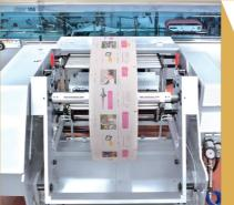
**Envelope Reel Unwinder** High capacity envelope unwinder for pre-printed or "white paper" digitally printed in-line.
