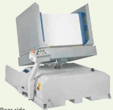
Rear side removal of bad sheets
